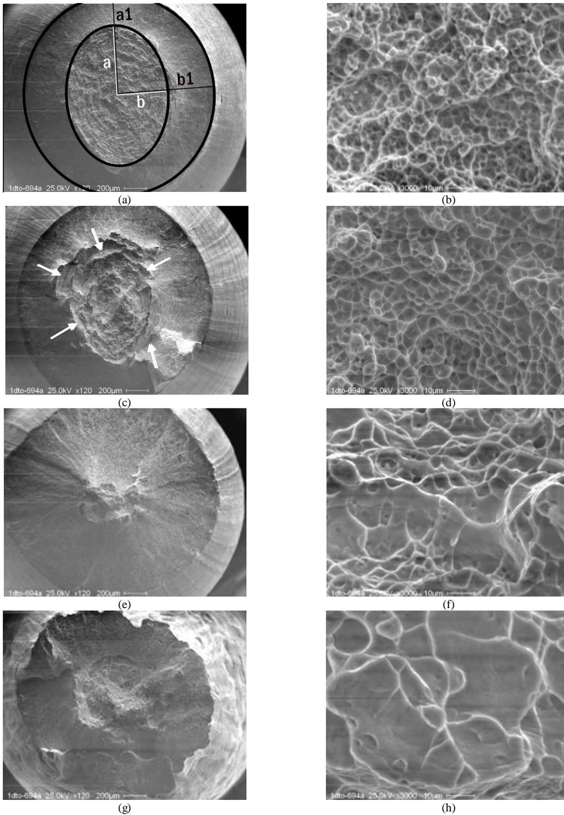
**FIGURE 1.** Fracture surface structure of VT16 samples solution treated at a, b – 725 °C; c, d – 775 °C; e, f – 850 °C; g, h – 875 °C for 1 hour and quenched.
