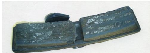
**FIGURE 2.** An exterior view of a composite brake shoe with the introduction of mass transfer plates
