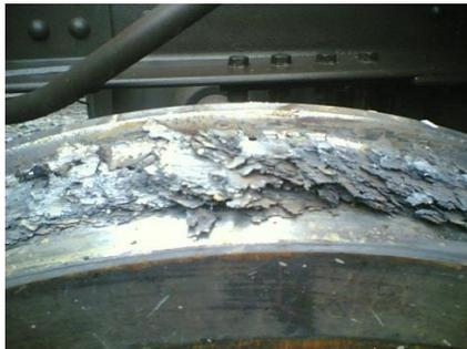
**FIGURE 1.** An exterior view of mass transfer plates on a decommissioned wheel
