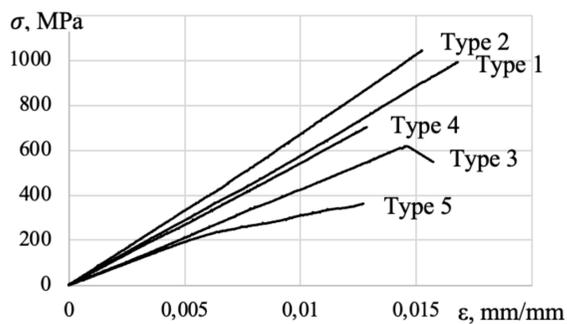
Fig. 2. Typical deformation diagrams of CFRP specimens of various reinforcement schemes during uniaxial tensile testing (according to ASTM D 3039)
