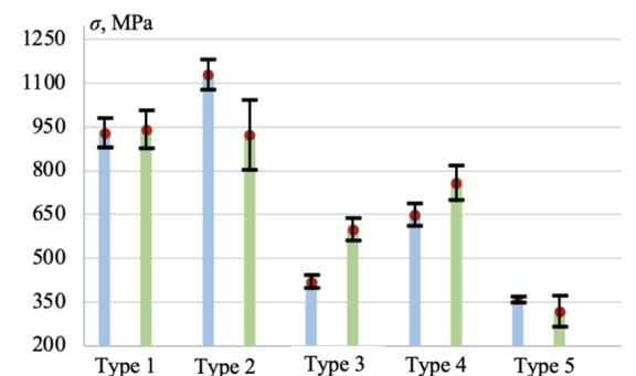
Fig. 4. Dependence of ultimate strength characteristics on the type of reinforcement of composite specimens: stress limit value according to ASTM ( $F_{OHTu}$ ) - blue line; solid specimen tensile strength ( $\sigma_B$ ) - green line
