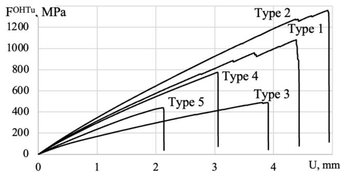
Fig. 3. Loading diagrams of CFRP specimens with an open hole in tension (according to ASTM D 5766) with different reinforcement schemes
