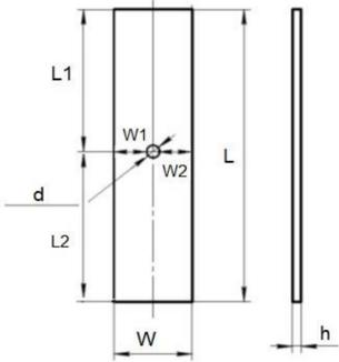
Fig. 1. Sketches of specimens with open-hole
