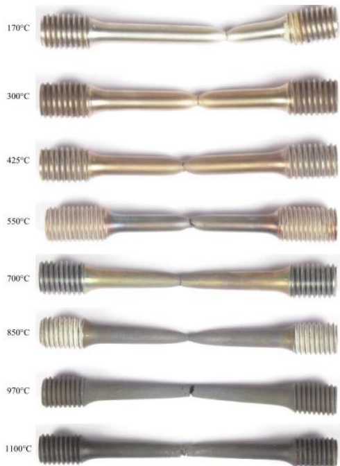
Tensile properties of SS 304L.
