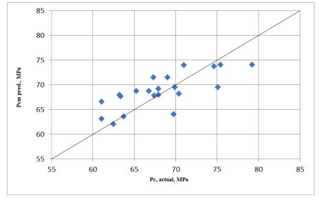
Figure 2 - Comparison of neural network prediction results and the actual tests results
