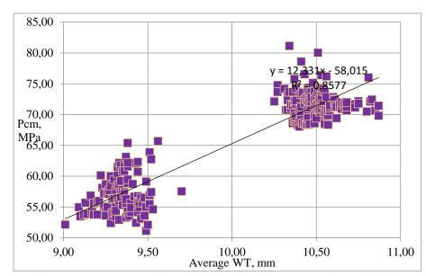
Figure 1 - Dependence of the collapse pressure value on the pipe wall thickness with an OD of 177.8 mm and with a wall thickness of 9.19 mm and 10.36 mm, grade P 110
